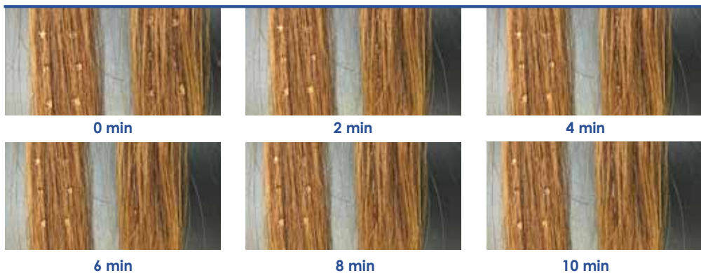
Figure 4: Absorption of water droplets into hair. Left: hair treated with 7% glycolic acid solution; Right: hair treated with 7% citric acid solution
